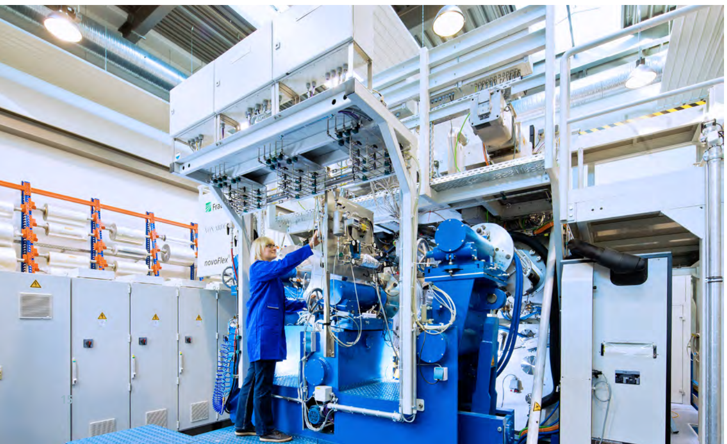
novoflex® 600 – Roll-to-roll pilot web coater
